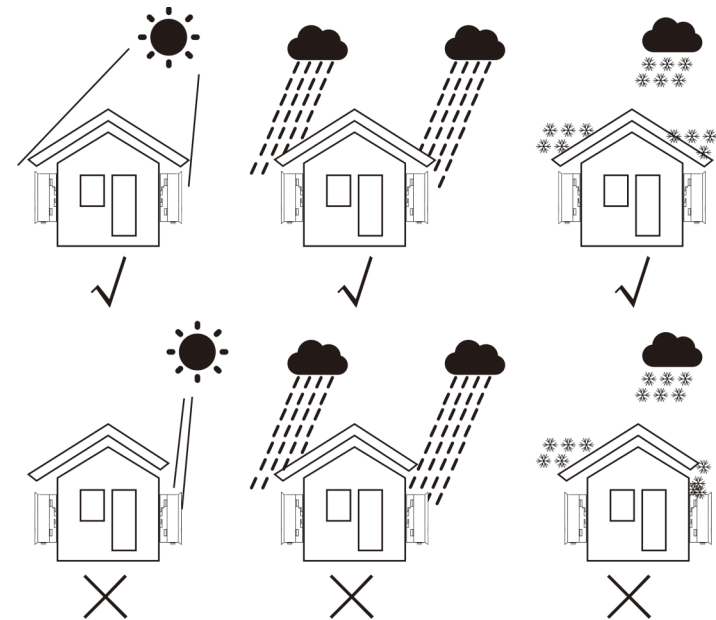
▲ Figure 5.1 Recommended installation position
